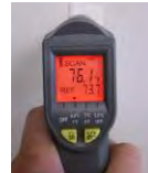
RED SCREEN TEMP. REACHES ABOVE SET TEMP.
